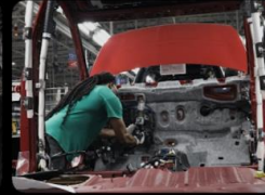
Brake pedal installation
