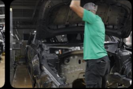
Hood lifter installation
