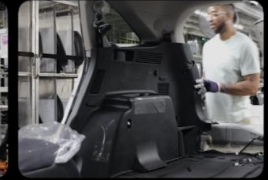
Luggage side trim loading & installation
