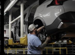
Wheel guard installation
