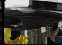
Underbody cover installation
